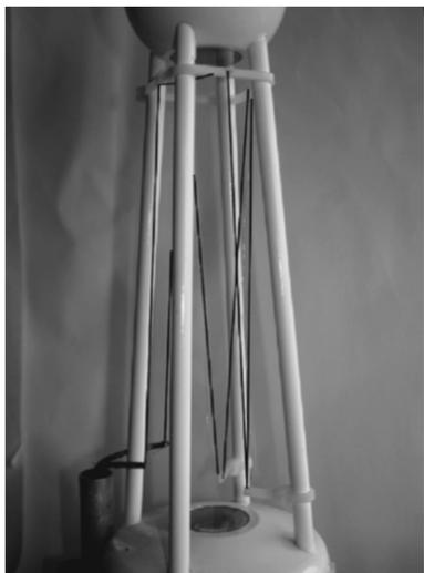
Grelle and Burba (2007) installed a fine wire PRT in the sensing volume of the open-path analyzer to measure the extra heat generated by the lower cylinder
