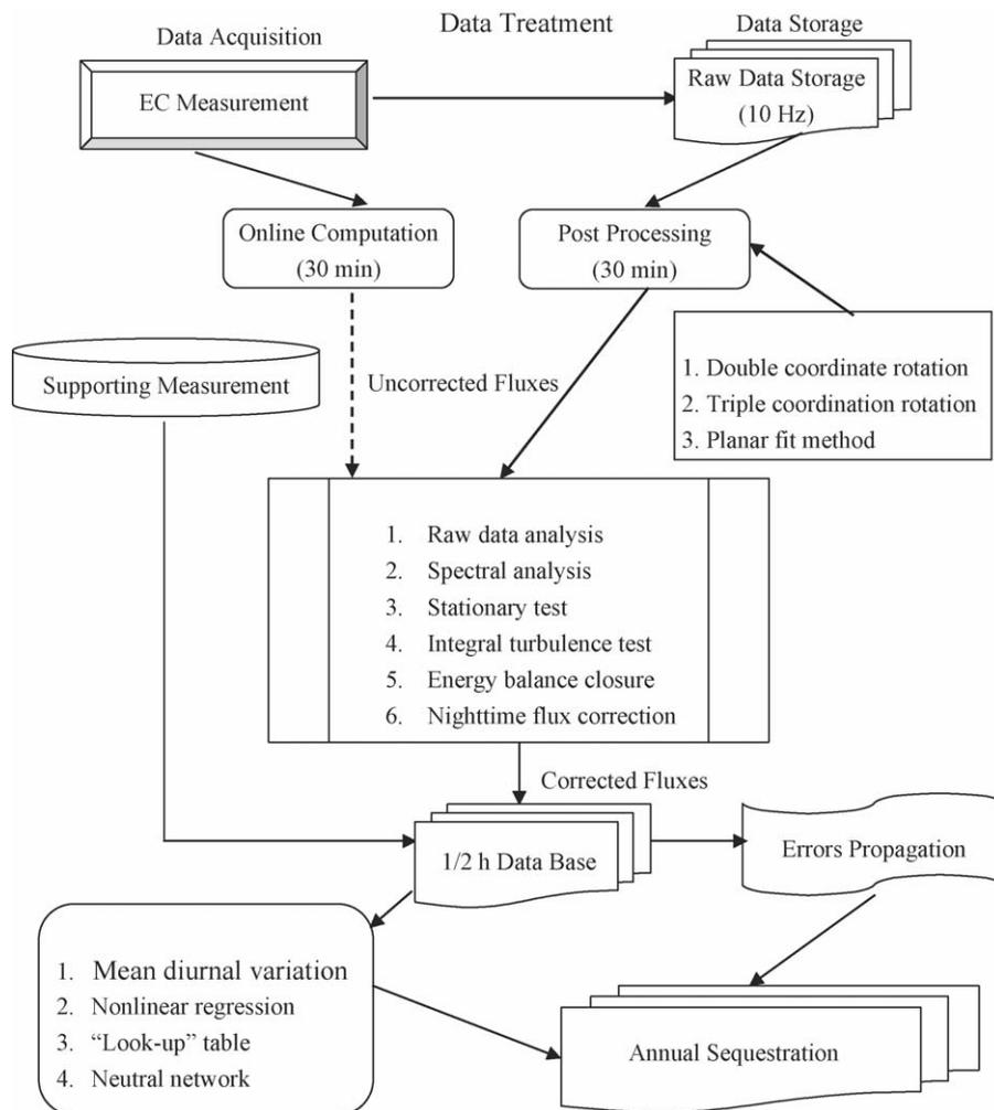
Fig. 3. Flow chart of data acquisition, processing and archiving. Dash line indicates that the online flux data will be used if the raw time series lost due to system failure.
