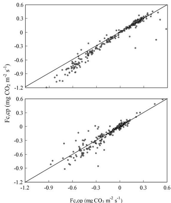
Fig. 4. Comparison of the CO<sub>2</sub> flux measured by the open-path ( $F_{c,op}$ ) and closed-path eddy covariance system ( $F_{c,cp}$ ) (a) before (22–28 June, 2003) and (b) after (20–26 October, 2003) system enhancement at QYZ forest site.
